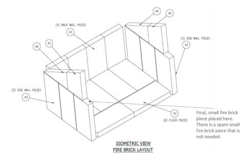
3. Finally, the T-bar retainer pieces (2) should be installed on both sides in order to keep the bricks in place.
