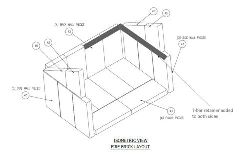
4. It is normal to have small gaps between the bricks upon completion. The bricks can be shifted towards the rear of the fire box.
