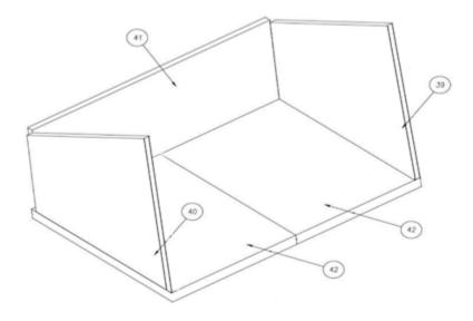
**Step 3:** Next, install the fire bricks. The first bricks to install are the four rear wall bricks and then the three bricks on the left and right side wall. A small gap may exist in between the corner of the bricks as shown in the diagram. Next, install the six bricks on the floor of Nova. Push all bricks up against the side and back walls. You may have a gap in the middle of the firebox as shown below. These can be filled with the brick slivers contained within your fire brick boxes.
