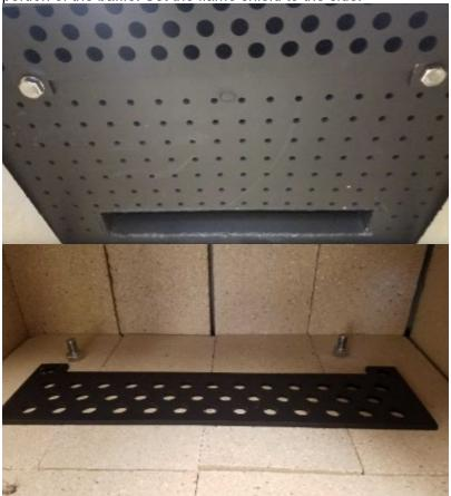
**Step 3:** Slide the catalytic combustor through the rectangular opening. The mesh sides should be facing the front and rear of the stove as shown in the diagram below.
