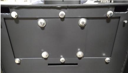
**Step 2:** Next, reach inside the back of the stove and remove the spacer plate and the flue collar, secured with 4 bolts and 2 washers each, located on the inside top of the stove.
