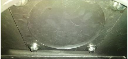
**Step 4:** Replace the access plate and install the flue collar, as shown below.
