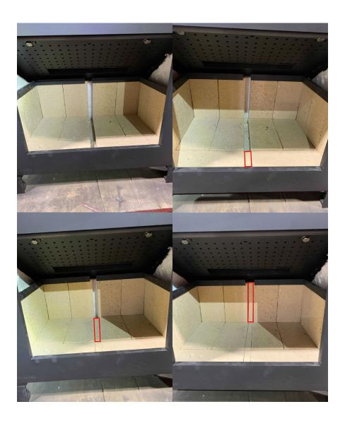
Lastly, the partial bricks that make up the second row of bricks on the side of the stove should be installed. To hold this row of bricks in place, the two T-bar retainers need to be inserted to both sides of the stove.
