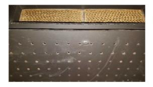
**Step 4:** Slide the catalytic combustor into the holding box, pushing back the combustor door, and sliding the combustor back as far as it can go in the holding box. The combustor may be a snug fit, which is normal.
