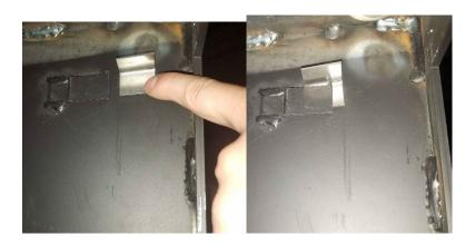
**Step 8:** To insert the removable ash tray, simply slide between the bottom of the stove and the top of the pedestal, as shown below.
