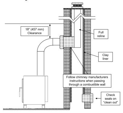
Special care must be taken regarding the wall thimble, or penetration from the chimney connector pipe to the masonry chimney, if the wall thimble must pass through a combustible exterior wall. Here all chimney manufacturer's instructions must be followed, including guidance on spacing to combustible surfaces, piping requirements, and liner requirements. Check with local authorities before installation to ensure all requirements are met.
