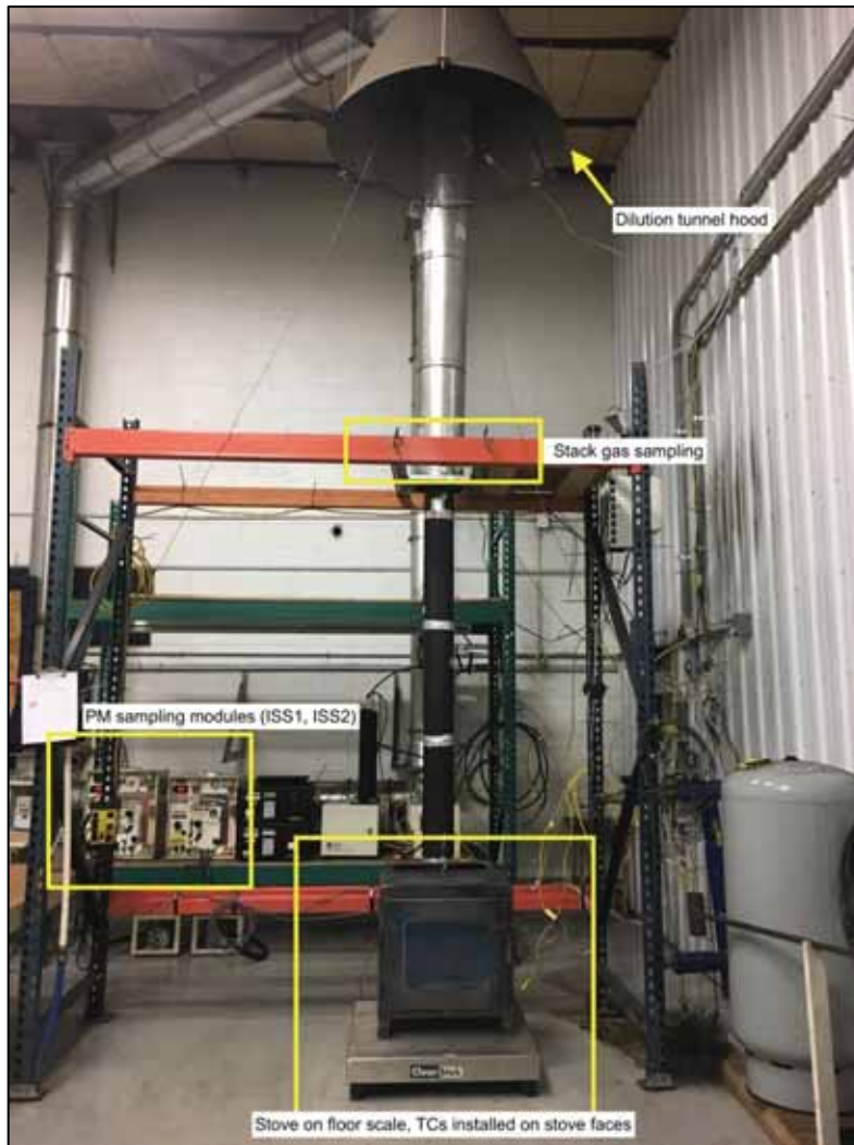
Figure 3. Stove installed on scale installed on test stand
