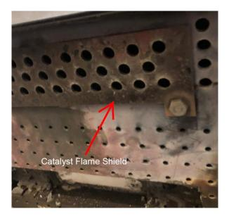
This was determined to be an oversight in setting the stove up for testing after shipment. This shield is a critical emissions component, so testing was halted, and the EPA contacted for approval to restart certification testing. With this approval, the shield was installed in accordance with the manufacturer's instructions and testing continued.
