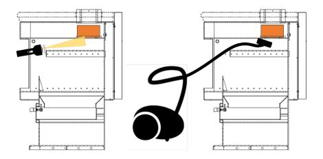
A properly functioning catalytic combustor maintains temperatures in excess of 500 °F. Following cleaning, the catalytic combustor does not function, it may need to be replaced. For replacement instructions refer to Catalytic Combustor Troubleshooting and Replacement section of this owner's manual.
