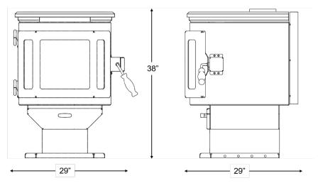
All clearances, side, corner, and back, are measured from the largest dimensions.
