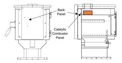
To access the catalytic combustor, first remove the back panel of the stove, then remove the catalytic combustor panel. The catalytic combustor (orange) may then be lifted up and removed from its ring holder. If any cracking or peeling is observed, the catalytic combustor must be immediately replaced. Please contact MF Fire for a replacement catalytic combustor.
