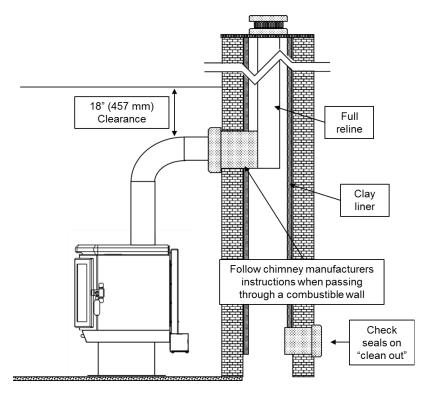
Special care must be taken regarding the wall thimble, or penetration from the chimney connector pipe to the masonry chimney, if the wall thimble must pass through an exterior wall. Here all chimney manufacturer's instructions must be followed, including guidance on spacing to combustible surfaces, piping requirements, and liner requirements. Check with local authorities before installation to ensure all requirement are met.
