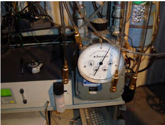
Picture 8 : Reference dry gas meter
